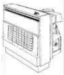
Gas fire and back boiler
